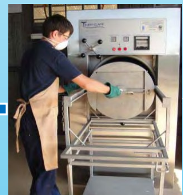
When finished, open the door and remove sterilized barrel
