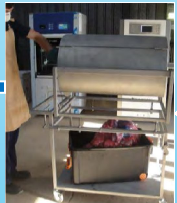
Unlock & rotate barrel to dump treated waste at the bottom
