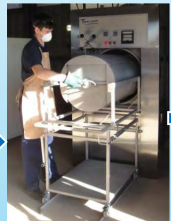
Slide barrel into autoclave
