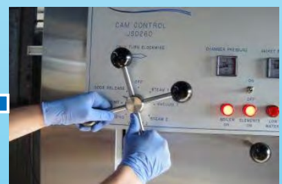
Start heating, multi-vacuum and sterilization cycles
